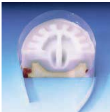
Cross-section of a flaskless duplicating mould
